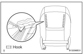
(c) Using a screwdriver, detach the 2 hooks.
