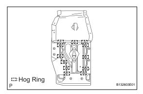
(e) Using hog ring pliers, install 12 new hog rings.
