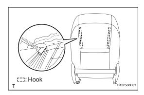
(f) Using hog ring pliers, attach a rubber with 3 new hog rings.
