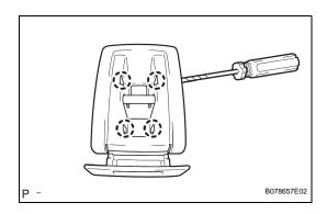
(d) Using a screwdriver, detach the 4 claws and remove the rear seatback cover.
