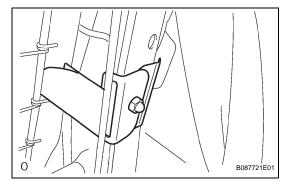
(d) w/ Front Seat Side Airbag:Fully cover the airbag with the 2 seatback cover brackets and install the nut.
