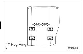
(i) Remove the 6 hog rings and seatback cover from the seatback pad.
