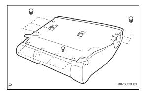
(g) Using a clip remover, remove the 9 clips. **NOTICE:**
