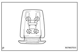
(g) Attach the 4 claws to install the rear seatback cover.
