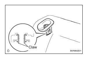
(e) Using a screwdriver, detach the claws and remove the seatback stop button grommet. HINT:
