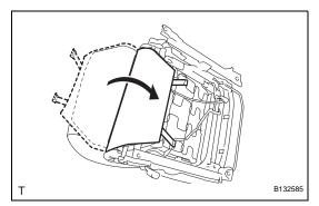
(c) Attach the 2 rubber bands of back of the front seatback cover.
