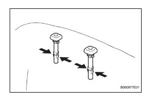
(c) Attach the 4 claws to install the 2 headrest supports.
