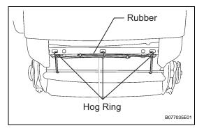
(g) Using hog ring pliers, install 3 new hog rings.
