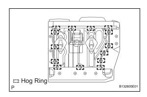
(e) Using hog ring pliers, install 14 new hog rings.
