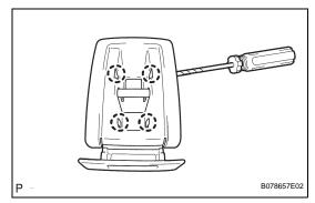
(f) Using a screwdriver, detach the 4 claws and remove the rear seatback cover.
