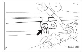
(e) Install the No. 1 parking brake cable to the floor with the clamp bolt.
