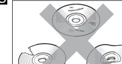
(a) Check that the map disc is not deformed or cracked.
