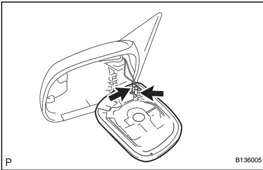
(b) Disconnect the 2 connectors and remove the mirror.
