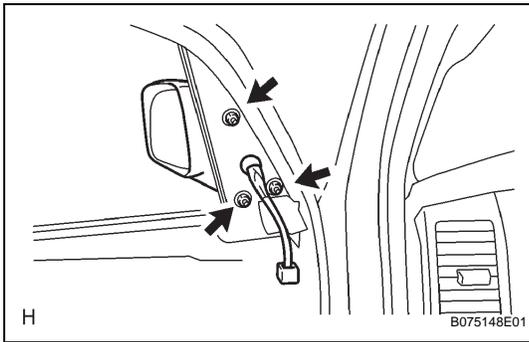
2. **INSTALL OUTER REAR VIEW MIRROR ASSEMBLY LH**
