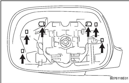
(c) Using a screwdriver, detach the 6 claws and remove the mirror cover.
