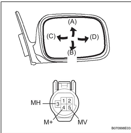
**2. INSPECT OUTER REAR VIEW MIRROR ASSEMBLY RH**
