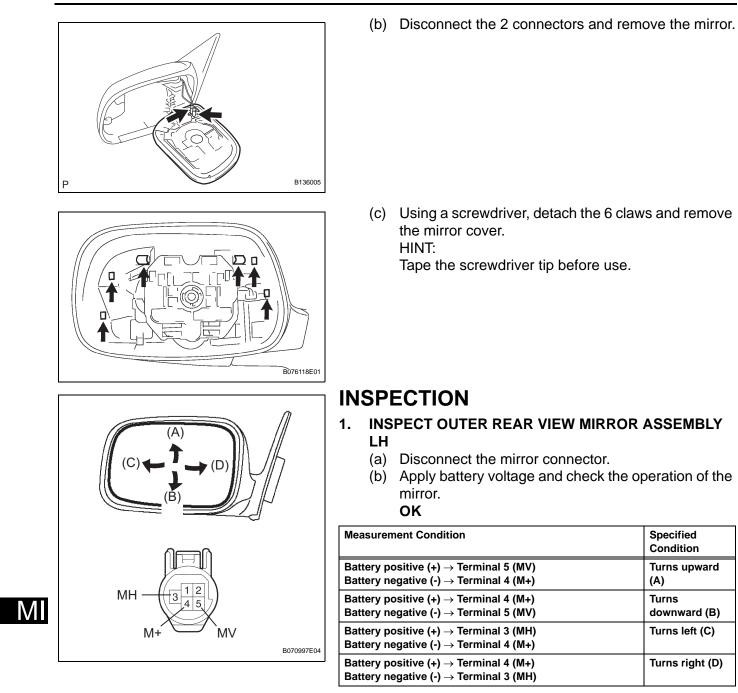
If the result is not as specified, replace the mirror assembly.
