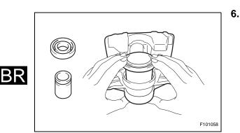
(c) Apply lithium soap base glycol grease around the front disc brake piston and install it to the front disc brake cylinder.
