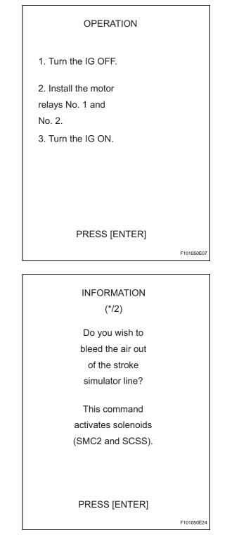
(c) Install the No. 1 and No. 2 motor relays.
