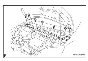
(c) Remove the 7 bolts and outer front cowl top panel.
