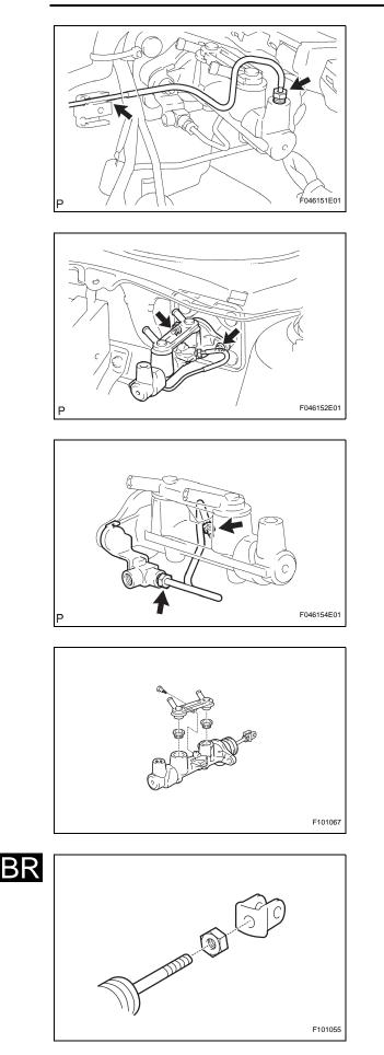
(f) Using SST, disconnect the No. 2 front brake tube from the clamp and brake master cylinder.
