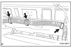
(b) Remove the 3 clamps from the outer front cowl top panel.
