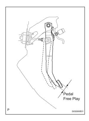
(5) Turn the stop light switch so that the clearance between its thread portion tip and the area where the pedal makes contact is between 0.5 to 2.4 mm (0.020 to 0.095 in.). Tighten the lock nut.
