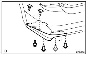
(3) Install the side spoiler with the 2 retainers, 2 clips and 3 screws.
