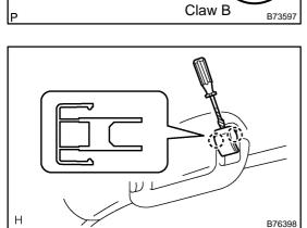
(b) Using a screwdriver, Disengage the 2 claws labeled A and 2 claws labeled B and remove the map lamp.
