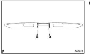
(c) Remove the 2 screws and back door opener switch from the garnish.
