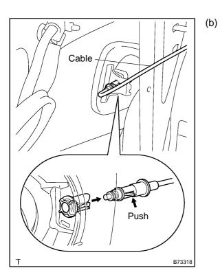
Disengage the claw and remove the cable.
