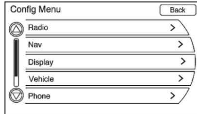
Press the CONFIG button to enter the menu options. Turn the TUNE/MENU knob to scroll through the available setup features. Press the TUNE/MENU knob or press the Display screen button to display other options within that feature.
