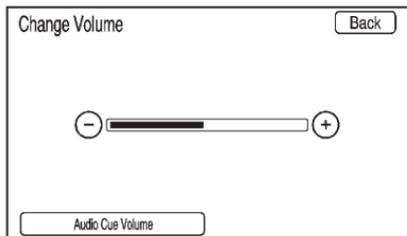
**Audio Cue Volume:** Press the + or – screen buttons to adjust the audio cue volume. The audio cue volume has a minimum volume. A “Limit Reached” pop-up will display when the volume has been changed to less than the minimum volume.
