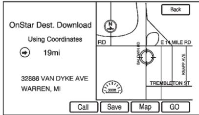
In this case, “Using Coordinates” displays on the downloaded screen.
