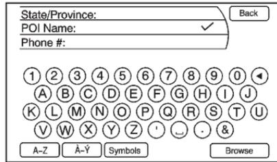
3. Enter the name or select by phone number. A list displays if four or fewer names are available. If there are more than four, there is a match counter with a number of available POI names. Press the List screen button to view the list.
