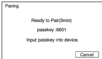
On the cell phone, locate the device named “Your Vehicle.” Follow the instructions given on the cell phone or follow the voice prompts, to enter the four-digit Personal Identification Number (PIN) that has been provided.
