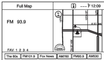
Press the source indicator button to display the current audio source screen. The display shows a split screen with the audio source screen on the left side and the map or guidance screen on the right side. Press the Full Map button to exit the split screen.
