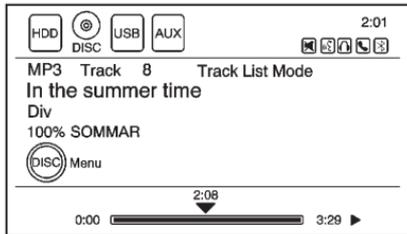
If a disc is already loaded, but you are currently on a map screen or listening to a different audio source, press the HDD/DVD/AUX button to switch to the disc source. A track number appears on the display when each track starts to play.
