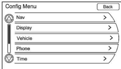
1. Press the CONFIG button. Turn the TUNE/MENU knob until the Phone menu displays. Press the TUNE/MENU knob or press the Phone screen button to display other options.
