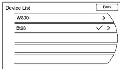
3. Turn the TUNE/MENU knob until Device List displays. Press the TUNE/MENU knob or press the Device List screen button to display other options.
