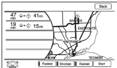
This menu displays if the symbol and waypoints are entered. Select the main map view to display the distance and time remaining from the current vehicle position to any of the set waypoints or final destination.
