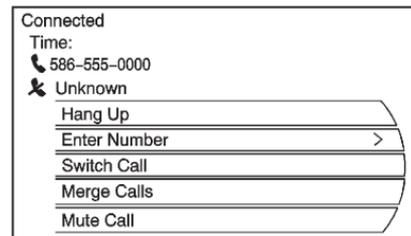
**Switch Call:** Turn or press the TUNE/MENU knob to Switch Call and press Enter or press the Switch Call option.
