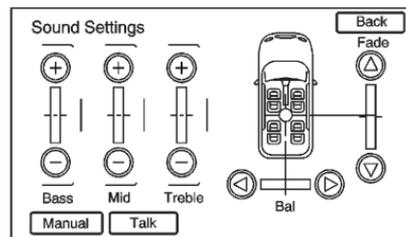
**EQ (Equalization):** The EQ settings are selected through the Sound menu. If the vehicle is equipped with the Bose® Energy Efficient Series sound system, EQ provides a choice of Manual or Talk settings.
