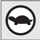
If this warning light illuminates, the power provided by the electric motor will be reduced and the vehicle will be only able to move at low speeds.
