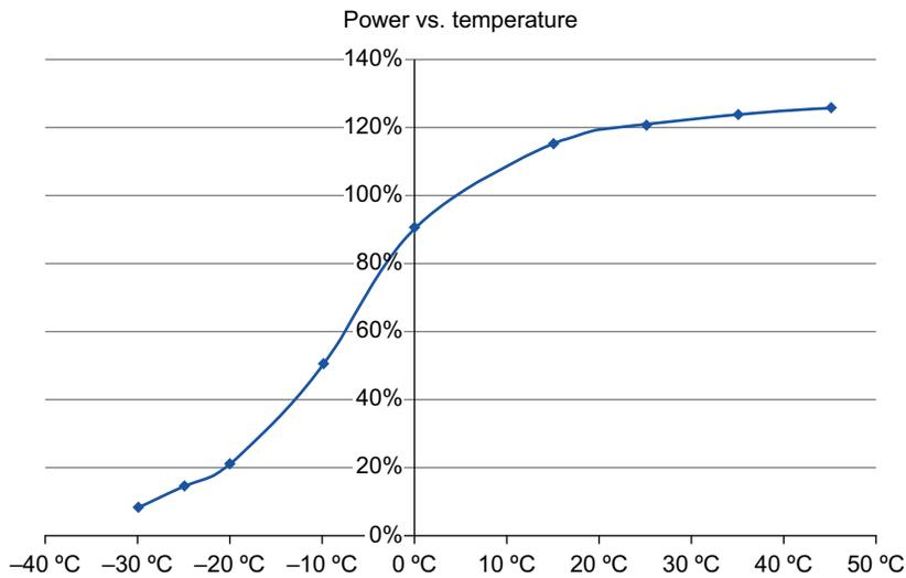
**FIGURE 8.15** Power as function of the lithium-ion battery temperature. (For color version of this figure, the reader is referred to the online version of this book.)
