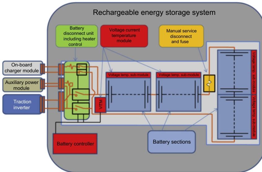
FIGURE 8.10 High-voltage architecture and details of the battery system. (For color version of this figure, the reader is referred to the online version of this book.)
