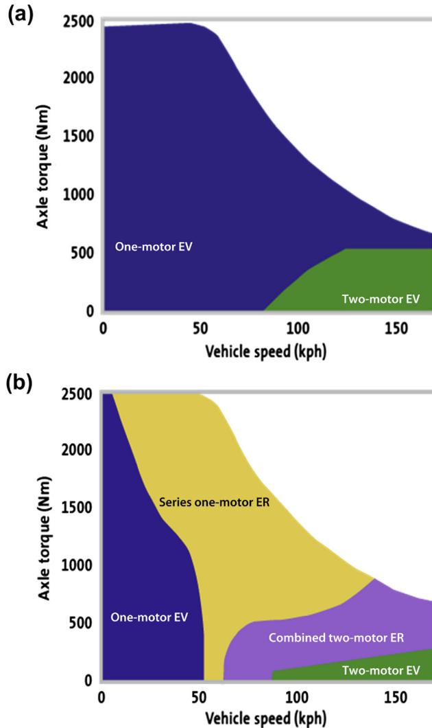
**FIGURE 8.12** (a) Pure EV; (b) extended-range drive operation. (For color version of this figure, the reader is referred to the online version of this book.)
