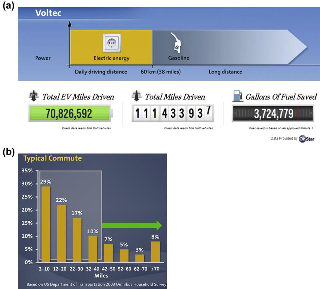
**FIGURE 8.20** (a,b) Share of driving in EV mode (Chevrolet Volt fleet in the United States, status as of July 31, 2012). (For color version of this figure, the reader is referred to the online version of this book.)
