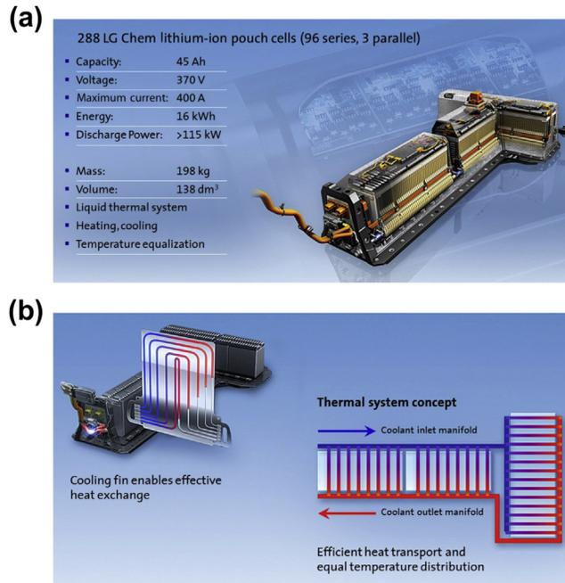
FIGURE 8.9 (a) Voltec battery pack; (b) active thermal system. (For color version of this figure, the reader is referred to the online version of this book.)
