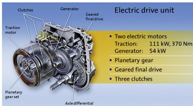
**FIGURE 8.8** Voltec electric drive unit. (For color version of this figure, the reader is referred to the online version of this book.)
