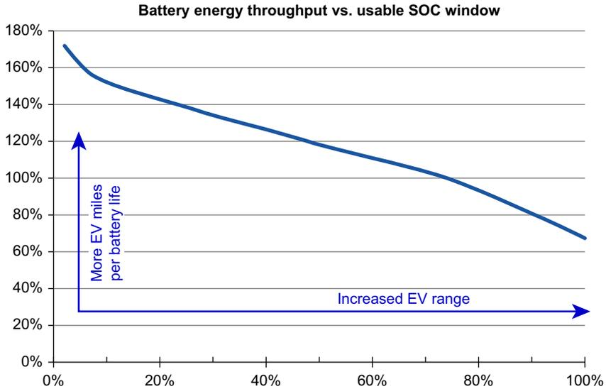
**FIGURE 8.14** Total battery energy throughput as function of the state-of-charge window size. (For color version of this figure, the reader is referred to the online version of this book.)
