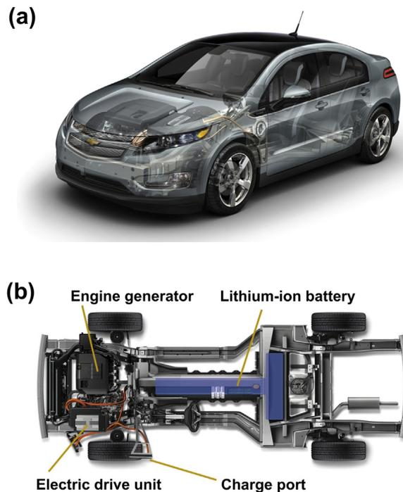
**FIGURE 8.5** (a) Chevrolet Volt; (b) the Voltec system. (For color version of this figure, the reader is referred to the online version of this book.)
