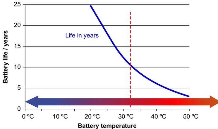
**FIGURE 8.16** Battery life is shorter at higher temperatures. (For color version of this figure, the reader is referred to the online version of this book.)
