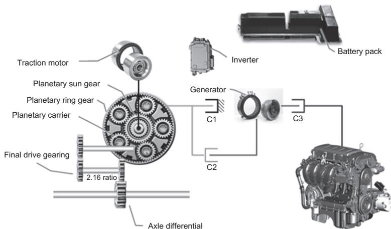
FIGURE 8.11 Voltec drive architecture with clutches and planetary gear set.
