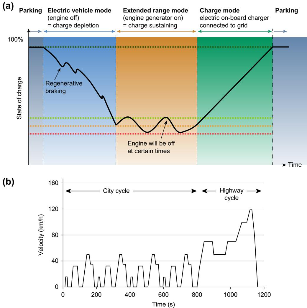
**FIGURE 8.6** (a) Operation modes of extended-range electric vehicles, from Ref. [5]. (b) New European Driving Cycle. (For color version of this figure, the reader is referred to the online version of this book.)
