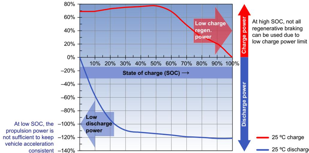
**FIGURE 8.13** Lithium-ion battery charge and discharge power. (For color version of this figure, the reader is referred to the online version of this book.)
