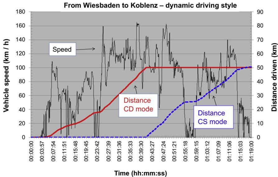
**FIGURE 8.18** Recording of a 50-km range in charge-depletion mode, real-world data (from Wiesbaden to Koblenz); dynamic driving style. (For color version of this figure, the reader is referred to the online version of this book.)
