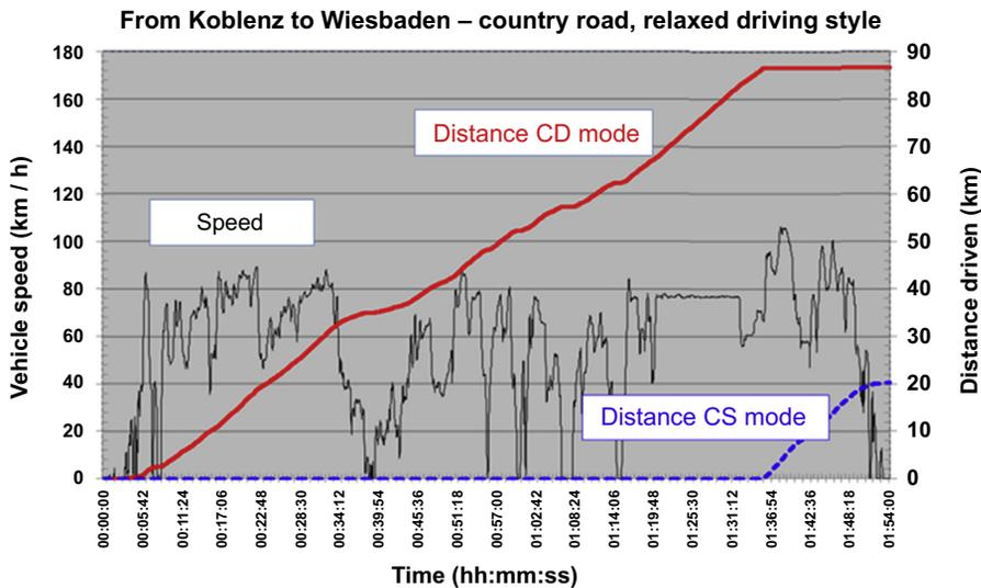
**FIGURE 8.19** Recording of a 86-km range in charge-depletion mode, real-world data (from Koblenz to Wiesbaden); relaxed driving style. (For color version of this figure, the reader is referred to the online version of this book.)
