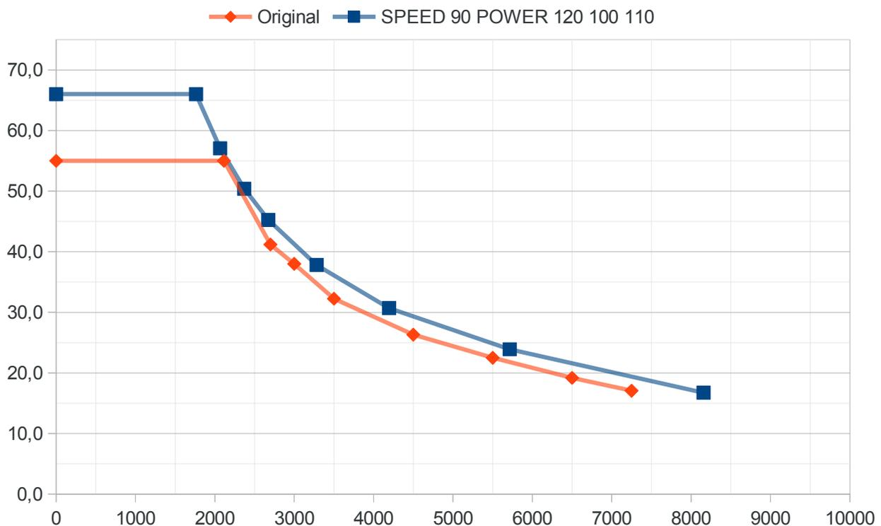
The original power map of the Twizy cuts back torque in the rpm range up to ~61 kph. It contains a nonlinearity, but one that does not look natural: if you take a look at 2700 and 3000 rpm, these do not fit into the overall curve, even if considering efficiency nonlinearity. Also, the mechanical power at the original turning point of 2115 rpm is 12.2 kW instead of the 13 kW. 13 kW will only be available from 5500 rpm upwards.
