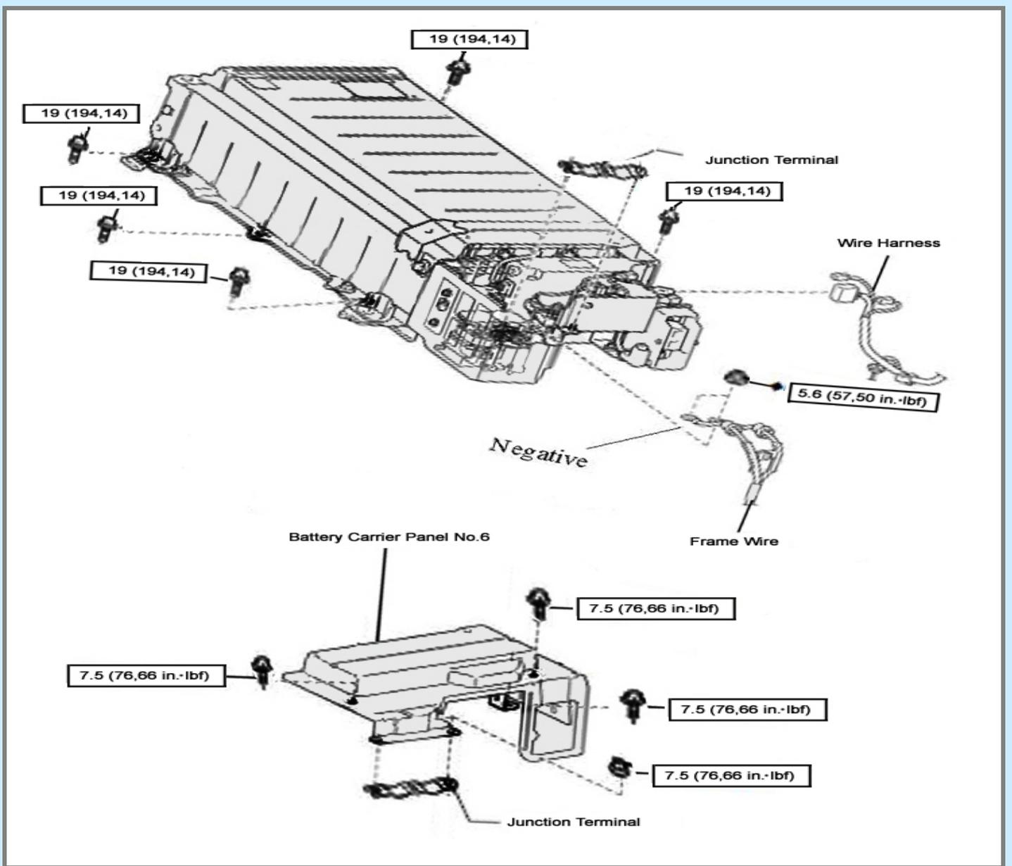
5. Connect the conversion kit's power cable to positive and negative terminals of the stock battery output power cable.
