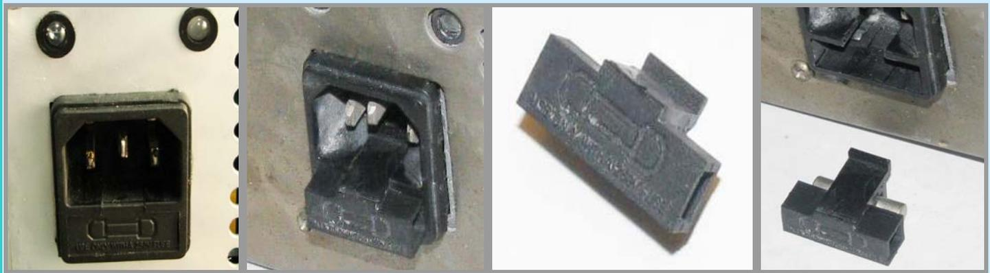
B. Converter fuse: The fuse block is connected to the high voltage wire. You can open the block by hand and replace the fuse.
