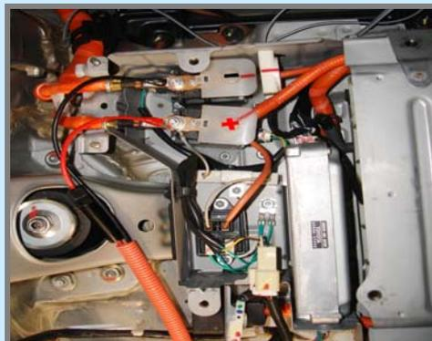
6. Install on/off switch panel.
