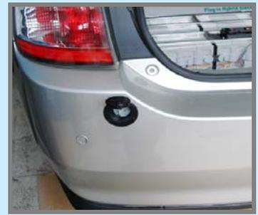
11. Install Charger's LED into the tail-light, this LED shows the performance of Charger:
