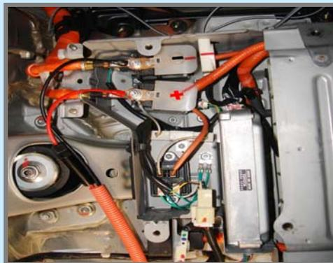
6. Install on/off switch panel.
