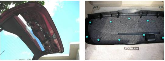
Above you can view the underside of the hatch with the panel removed and on the right, the friction lock pins on the underside of the panel which hold it in place. Next, remove the license and license plate holder from your hatch and discard the original screws. They will be replaced by the high security screws included in your kit. Configure your camera so that the camera body itself is located on the bottom of the frame (instructions are included in the
