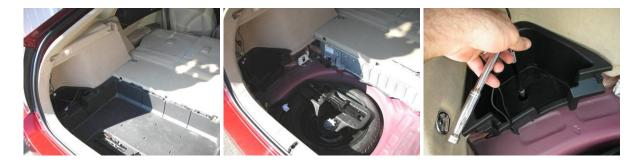
With the rear seat folded down, bring the video cable up to the battery cover panel. Remove the bolt on the tie down plate to allow the cable to be brought underneath. Pull the Velcro free from the back of the seat and pull the friction lock free from the corner to allow the cable to be fully hidden.
