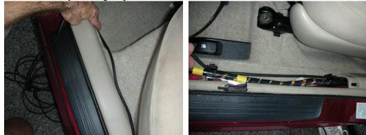
Finish your installation by bringing the video cable up to the back of the screen and plugging it into the connector provided by the Camera Lockpick. Tie up any extra cable and place behind the kickpanel before reinstalling.
