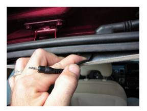
Plug in the matching Hitchcam harness to the camera cable and prepare to bring the other end down to the taillight assembly. Begin by removing the 10mm bolt on the rear panel and pulling the top edge out enough to tuck the wire in around the top edge. Remove the small panel over the taillight connections and pass the wire down through the opening.
