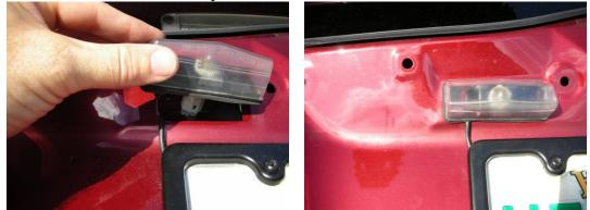
Press the light back into position and begin routing the wire to the hinge area. Press the wire underneath the edge of the plastic panels. Remove the panel from the underside of the hatch which is covering the latches to allow greater access. Again, the panel is not held in place by any screws and is simply pulled free from the friction locks underneath.
