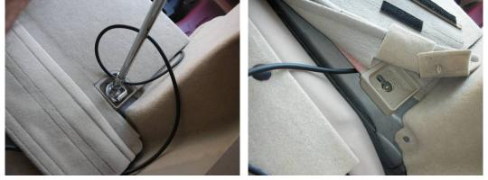
Bring the cable into the rear seat area. Pull up the front left corner of the rear seat bottom to allow the cushion to be lifted slightly. This allows you to tuck the cable underneath.
