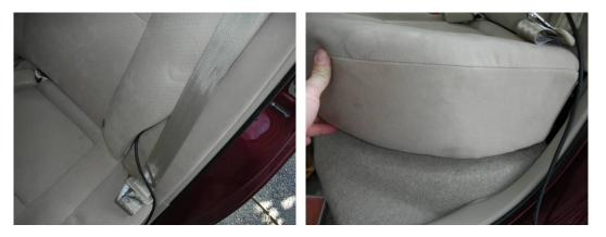
Tuck the wire under the edge of the trim panels along the doors as you bring the video cable up to the front of the car. The trim panel should be pulled up at the driver area to allow the kickpanel up front to be pulled free. Again, no screws are holding these panels in place and are simply pulled free with your fingertips.
