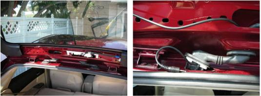
Lift up the rubber gasket around the hatch opening and pull down the edge of the headliner enough to retrieve the camera wire as you pass it into the car opening.
