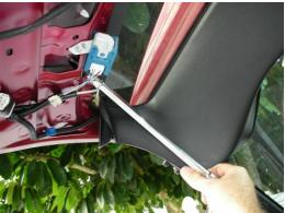
From the backside of the hatch, press the drivers' side license plate light assembly out of the hatch to allow the Camera cable to be passed underneath and into the inside of the car.
