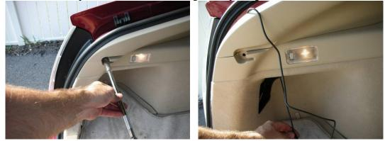
The wiring harness for your camera contains connectors and wire taps so that no wires will need to be cut during installation. The wire taps are designed to simply fold around a wire, and when squeezed together with a pair of pliers, create a convenient connection for your harness wires to plug into. Locate the wires behind the clear reverse tail light. Place wire taps on both wires of its connector (RED W/BLUE stripe and WHITE W/BLACK STRIPE )
