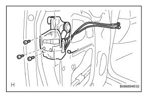
(d) Apply adhesive to the threads of the 3 screws. **Adhesive:**
