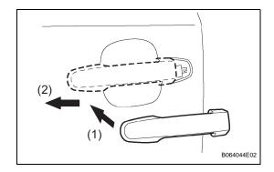
(c) Install the handle by pushing it in the direction of the arrow marks in the illustration.
