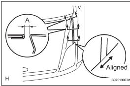
(b) Adjust the cushion rubber so that the height of the hood and the fender are aligned.
