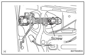
(b) Using a T30 "torx" wrench, loosen the screw of the frame.
