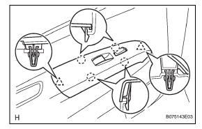
(g) Attach the 2 clips and 4 claws to install the armrest upper base panel together with the 2 switches.
