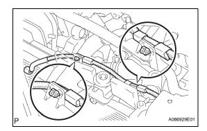
(r) Disconnect the wire harness clamps shown in the illustration.
