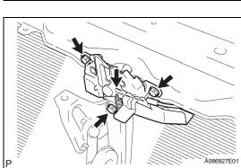
(o) Remove the 3 bolts, disconnect the hood lock control cable, and then remove the hood lock.
