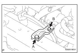
(h) Install the cooler bracket with the 2 bolts.
