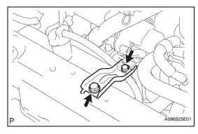
(m) Remove the 2 bolts and cooler bracket.
