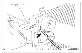
(g) Connect the horn connector shown in the illustration.
