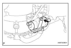
(c) Remove the bolt and coolant heat storage water pump.
