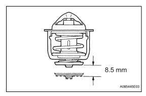
(c) Check the valve lift.
