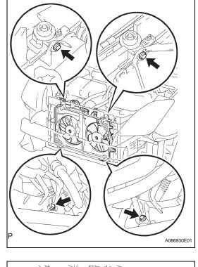
(b) Connect the 2 wire harness clamps shown in the illustration.
