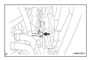
(e) Disconnect the connector shown in the illustration.
