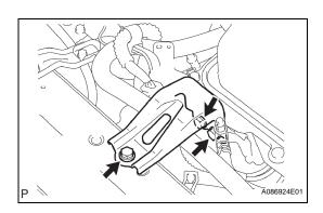
(I) Remove the 3 bolts and inverter bracket.
