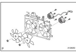
14. REMOVE NO. 2 COOLING FAN MOTOR(a) Remove the 3 bolts and fan motor.
