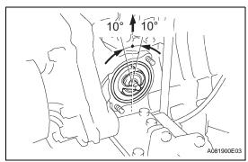
(b) Install the thermostat with the jiggle valve facing upward.
