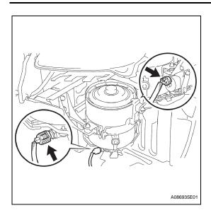
(b) Disconnect the water pump motor and temperature sensor connectors.
