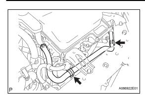
(I) Connect the inverter reservoir hose to each clamp.
