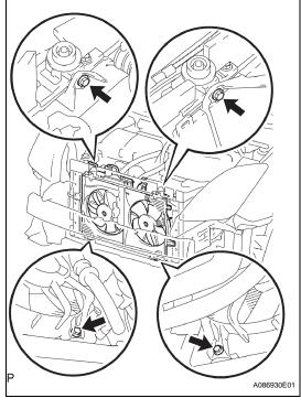
(s) Remove the 4 bolts, then remove the fan with motor from the vehicle.
