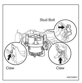
(d) Separate the stud bolt and 2 claws shown in the illustration, then remove the coolant heat storage tank.
