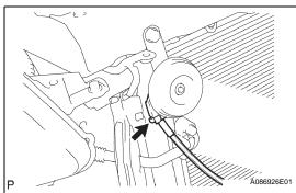
(n) Disconnect the horn connector shown in the illustration.
