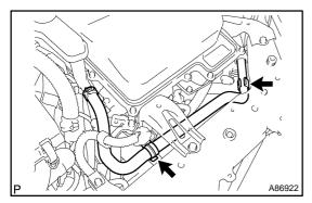
(I) Connect the inverter reservoir tank to each clamp.
