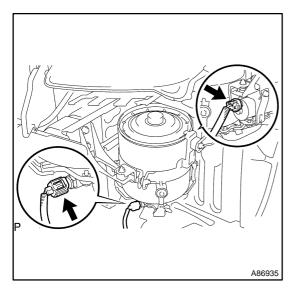
(c) Connect the 2 connectors of the water pump motor and temperature sensor.
