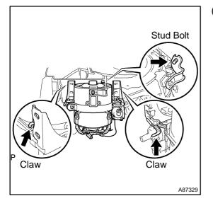
(d) Separate the stud bolt and 2 claws shown in the illustration, then remove the coolant heat storage tank assembly.
