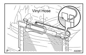
(d) Connect a vinyl hose to the bleeder plug of the radiator assembly and the radiator reservoir tank.
