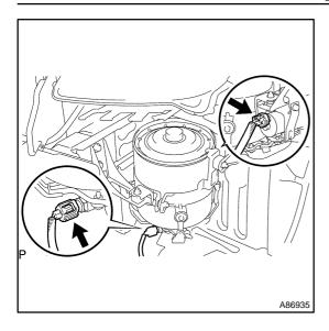
(b) Disconnect the 2 connectors of the water pump motor and temperature sensor.
