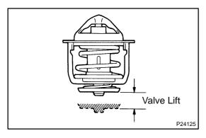
(c) Check the valve lift.
