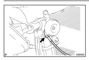
(g) Connect the horn connector shown in the illustration.
