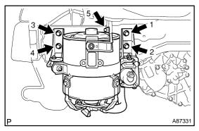
(b) Tighten the 4 bolts and nut shown in the illustration.
