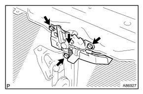
(o) Remove the 3 bolts and disconnect the hood lock control cable, then remove the hood lock assembly.
