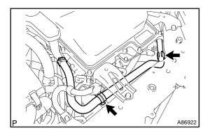
(i) Disconnect the inverter reservoir tank hose from the clamps.
