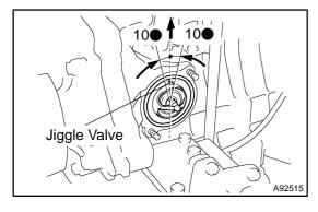
(b) Install the thermostat so the jiggle valve faces upward. HINT:
