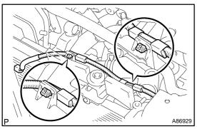
(b) Connect the 2 wire harness clamps shown in the illustration.
