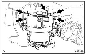
(c) Remove the nut and 4 bolts shown in the illustration. **NOTICE:**
