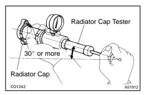
(a) Using a radiator cap tester, slowly pump the tester and check that the air is coming form the vacuum valve.
