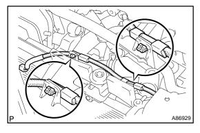
(r) Disconnect the wire harness clamps shown in the illustration.
