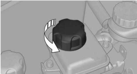
2. Slowly add coolant up to the specified level; do not overfill.
