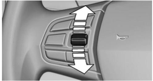
Press the rocker switch while the system is interrupted.
