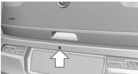
The camera lens is located underneath the tailgate. The image quality may be impaired by dirt.
