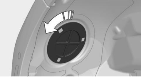
In the wheel house, turn the cover counter-clockwise and remove it.
