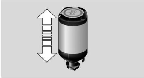
2. Take the connection hose completely out of the compressor housing. Do not kink the hose.
