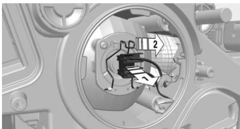
4. Press bulb holder slightly inward, loosen it to the right from the anchor and fold it down.
