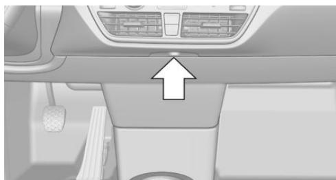
The socket is located underneath the instrument panel. Remove the cover.
