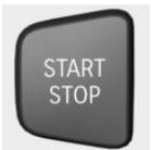
Pressing the Start/Stop button switches drive readiness on or off.
