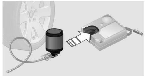
5. Screw the connection hose onto the tire valve of the defective wheel.
