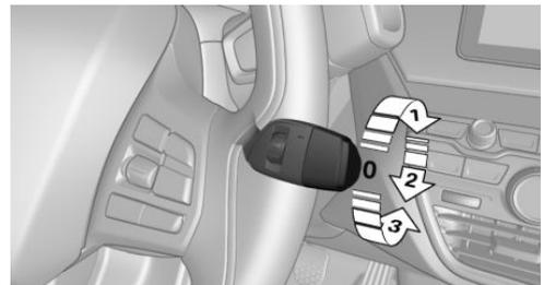
Turn the switch from idle position 0 upward, arrow 1: interval mode. When reverse gear is engaged, the system switches to continuous operation.
