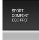
Pressing the button displays a list of the selectable programs. Depending on your vehicle's optional features, the list in the instrument cluster can differ from the illustration shown.
