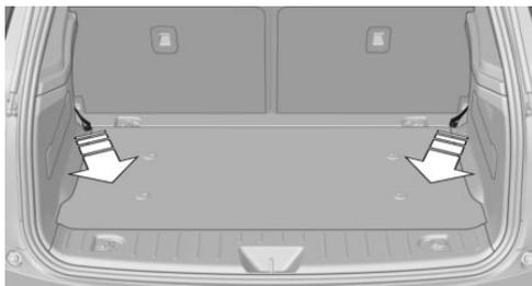
Or: pull the corresponding loop in the cargo area and fold the seat backrest forward.
