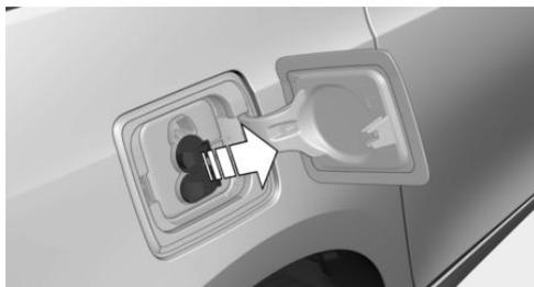
3. Connect either a Level 1 or Level 2 charging cable to the household socket or the port on the charging station.
