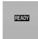
The READY display indicates that the vehicle is ready for driving. Drive readiness in detail, refer to page 65.
