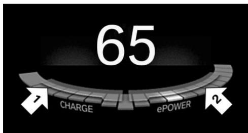
The energy recovery occurs during coasting and braking and is displayed in the performance display by the accelerator pedal indicator.
