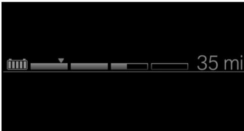
∇ The arrow on the charging state indicator designates the Range Extender reel-on time. If Range Extender is activated, the current charging state of the high-voltage battery is maintained.
