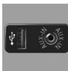
An external audio device, e.g., an MP3 player, can be connected via the AUX-IN port or the USB audio interface between the seats.
