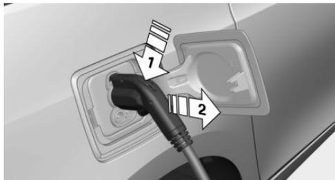
3. Remove the charging cable from the charging port, arrow 2.
