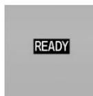
The READY display indicates that the vehicle is ready for driving.
