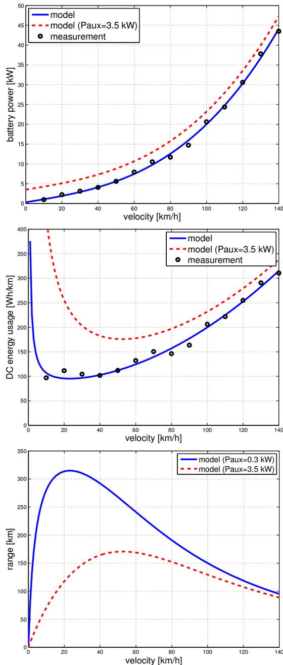
Figure 2: Battery power, DC energy usage and range as a function of forward velocity.
