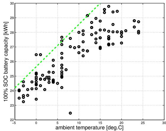
Figure 10: Calculated battery capacity using energy usage and SOC change for commuting trips.
