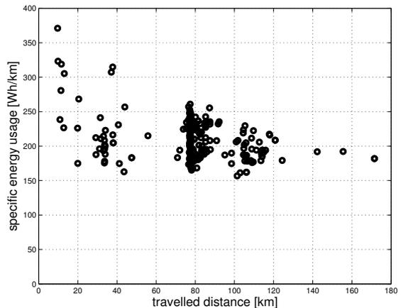
Figure 5: Specific energy usage as a function of trip length.
