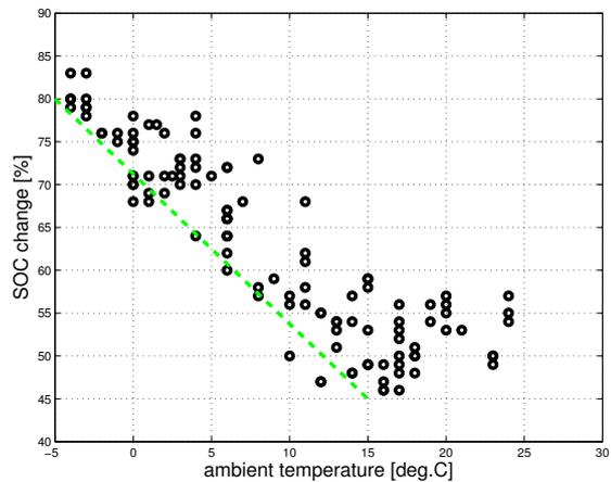
Figure 9: SOC change for different ambient temperatures while executing 77 km commuting trips.
