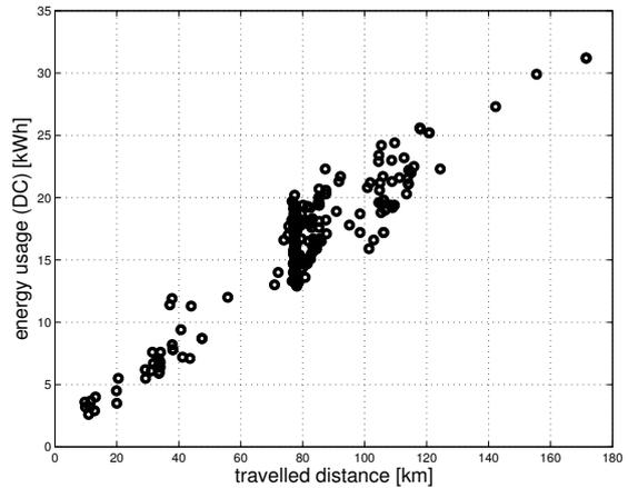
Figure 4: Energy usage as a function of trip length.
