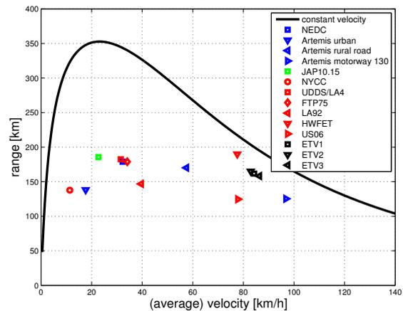
Figure 14: Vehicle range for various driving cycles (optimistic scenario, 15 °C).
