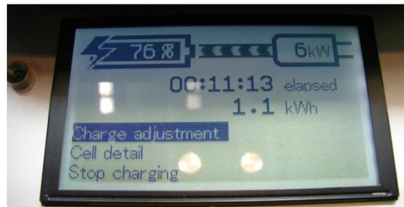
Figure 3: BMS display (during charging).
