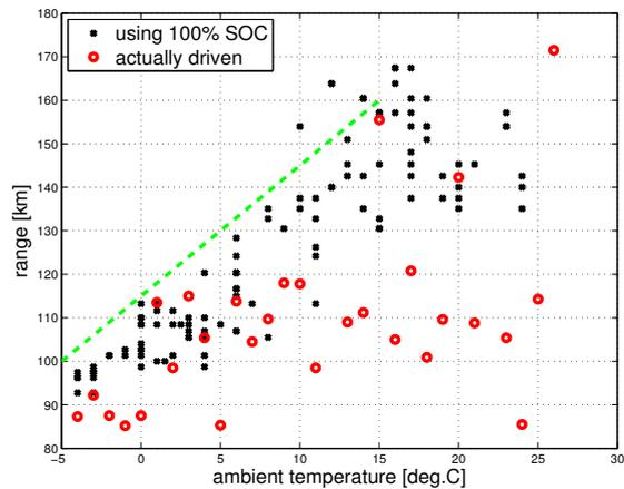
Figure 11: Calculated vehicle range using 100% SOC and actually driven distances.
