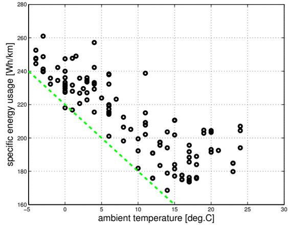
Figure 8: Temperature dependency of specific energy usage for commuting trips.
