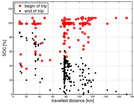
Figure 7: SOC at start and end of a trip.
