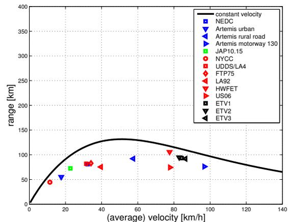
Figure 15: Vehicle range for various driving cycles (pessimistic scenario, -5 °C).
